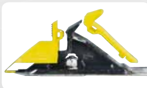
CLAMPS inside and outside fully protected with plastic protectors to avoid damaging the more delicate rims.
